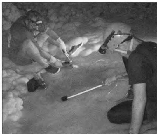
Figure 1. A diaphragm hand pump was adapted by Jim Werker for removing silt from the Pellucidar pools. (Lechuguilla's drip water had washed muddy footsteps across the flowstone and into pools where the silt settled on the bottoms.) Pool water is filtered through sponge material stuffed into a clean, cut-off water bottle. Dave Hamer is operating the pump to filter and circulate water back into the pool. (See page 12 of color section.)
