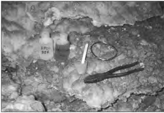
Figure 2 (Versamid) and Figure 3 (TETA). Epon 828 epoxy mixed with Epi-cure 3234 (TETA) curing agent in a 12:1 ratio is a relatively safe adhesive for cave applications. The Epon and Epi-cure products are manufactured by the Shell Chemical Company and are available through regional chemical or plastic product suppliers. Versamid hardeners are also used with Epon 828. For speleothem repair, always have mixing cups, mixing sticks, and disposable gloves on hand. To ease handling the products in a cave, premeasure both the epoxy and the hardener into small containers.
