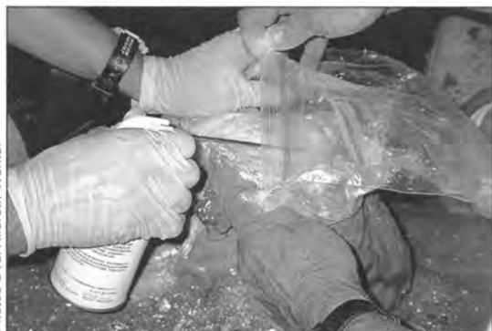
Figure 3. Compressed air in a can is handy for removing drill dust if the dust can be captured in a plastic bag.
