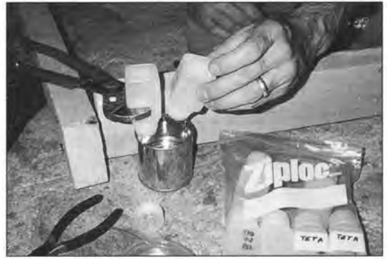
Figure 2 (Versamid) and Figure 3 (TETA). Epon 828 epoxy mixed with Epi-cure 3234 (TETA) curing agent in a 12:1 ratio is a relatively safe adhesive for cave applications. The Epon and Epi-cure products are manufactured by the Shell Chemical Company and are available through regional chemical or plastic product suppliers. Versamid hardeners are also used with Epon 828. For speleothem repair, always have mixing cups, mixing sticks, and disposable gloves on hand. To ease handling the products in a cave, premeasure both the epoxy and the hardener into small containers.
