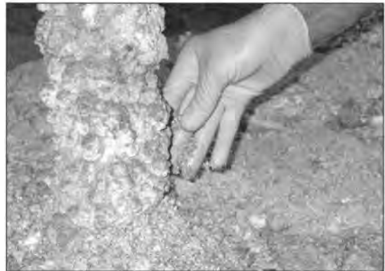
Figure 4. The outer crust of the base was reinforced with museum-grade epoxy mixed with calcite dust.
