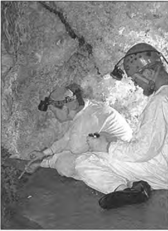
Figure 2. To collect water samples from a pristine cave pool, Penny Boston and Mike Spilde wear Tyvek suits, hair covers, surgical gloves, and flowstone shoes.
