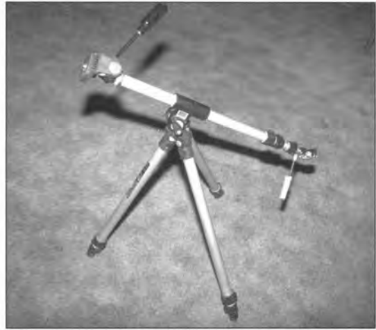
Figure 3. Use a basic photographic tripod that has a reversible periscoping center leg. Adapt the tripod to use with camera plates, adjustable pads, and rock-filled counterbalance bags.
