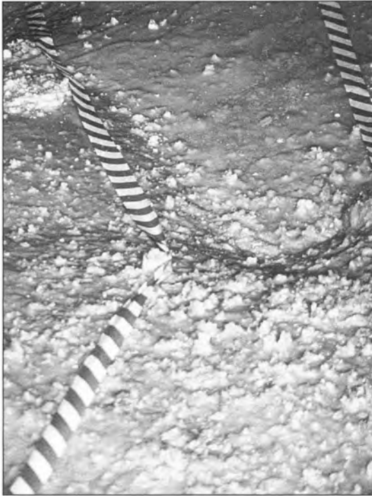
Figure 11. To avoid color bleeding, use white-backed flagging on wet flowstone surfaces. Surveyors' flagging tape is best secured on small natural protrusions. Red/white striped flagging may indicate delicate zones outside of the trail-marking tape.
