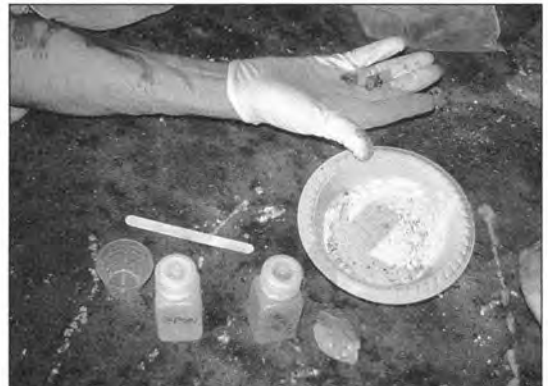
Figure 6. Pulverized rocks and archival epoxy form a thick, color-matched mixture for filling cracks and gaps in repaired speleothems.
